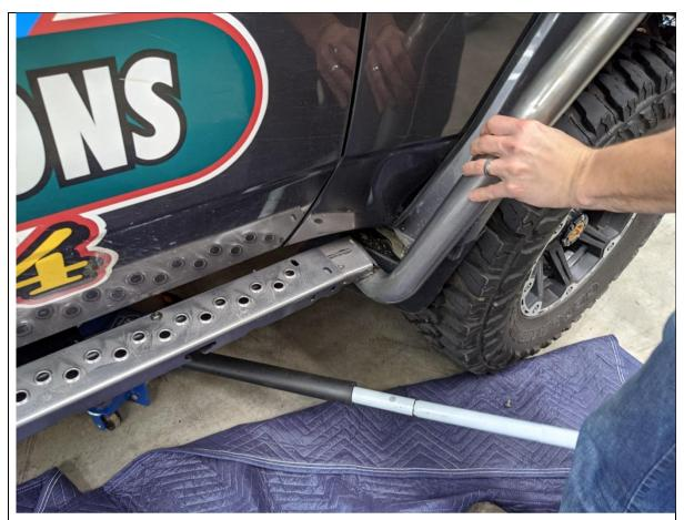
6. Fit the side rail to the slider by sliding it in from the front as shown.
