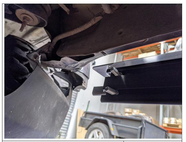
5. Fit 2x M10x25 Bolts (Contained in Rock Slider Kit) to the T slot in the extrusion as shown.
